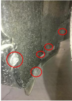
5. Remove the three 10mm bolts located at the bottom of the bumper skin.
