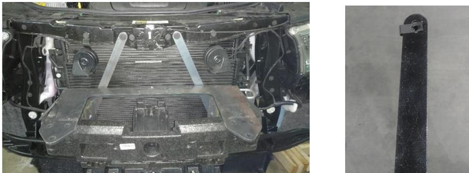
15. Trim brake duct work and rear bumper skin mount as shown in the photo. Trim duct work 4 1/2" and 7 1/2" (see picture).
