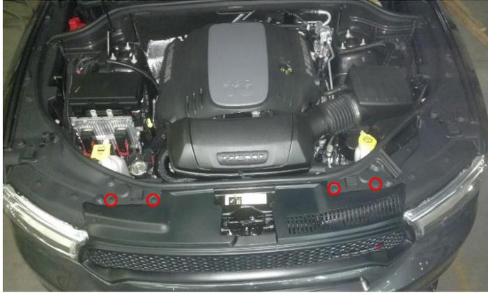
2. Remove the 2 plastic rivets and the 10mm bolt at each wheel well.
