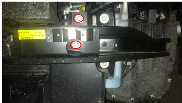
12. Remove the two 8mm bolts that attach the lower support struts.
