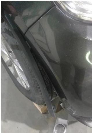
4. Remove the five 8mm bolts that attach the wheel well liner to the front bumper skin.
