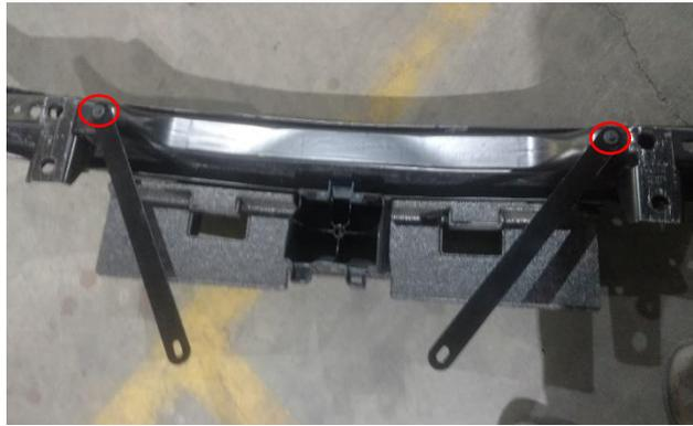
13. Trim plastic radiator duct work as shown. Reinstall internal bumper by starting at the bottom bolt and setting upper mount on to the started bolts and tighten bolts back to original position.
