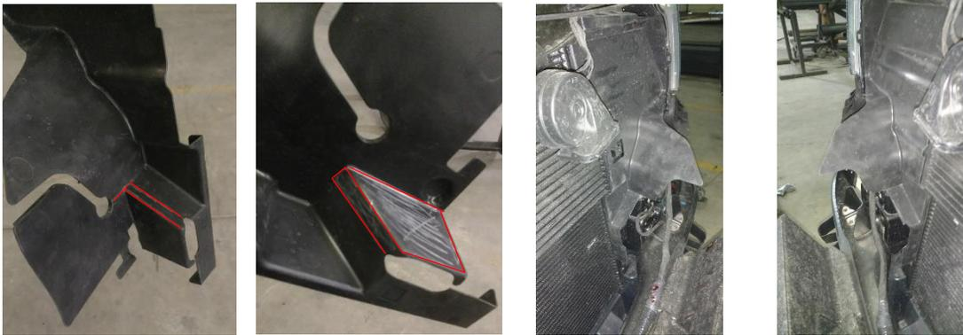
14. Install new radiator support struts attaching to the upper mount, using the provided 1/2" hardware on lower end of strut.
