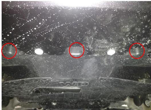
6. Remove the two 13mm bolts that hold the front of the transmission skid plate.
